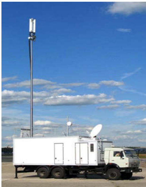
1-rasm. Mobil uyali stantsiya “Kamaz” rusumli avtoyuk moshinasining ko’rinishi.
